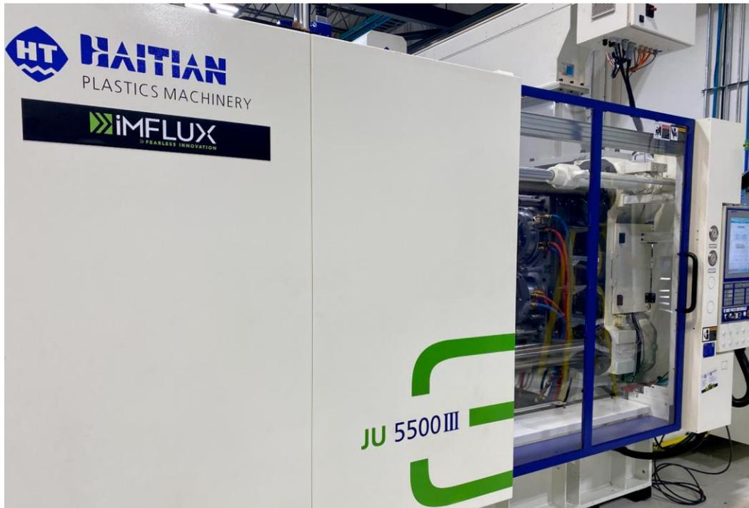
The iMFLUX technology center in Hamilton, Ohio hosts a 618-ton (U.S.) Haitian Jupiter III two-platen, servo-hydraulic press. The JU5500 III features iMFLUX technology as a result of a recently announced partnership with Absolute Haitian for customers in the U.S. and Canada.
