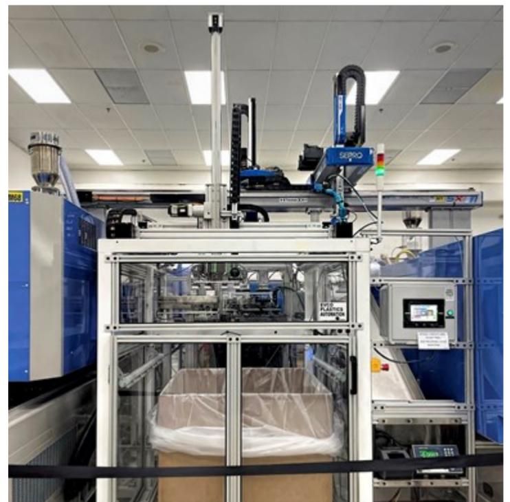
EVCO’s automation team is busy with projects like this consumer-packaging cell that ties together two injection presses with 16-cavity stack molds to produce mating parts that are conveyed, snapped together, packaged, labeled and inspected, after which data on each assembly is read via barcode and uploaded to a production and quality database in the cloud.
