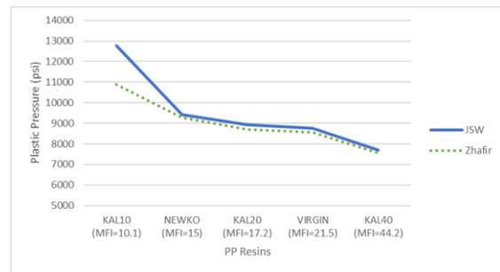
**Figure 20:** Inner barrel validation's average peak pressures of each material to make the same part process.
