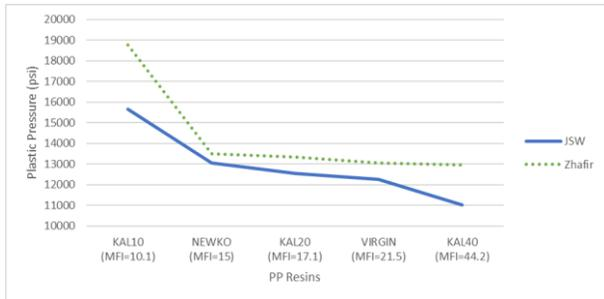
**Figure 21:** Outer barrel validation’s average peak pressures of each material to make the same part process.
