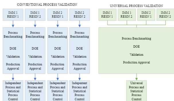
**Figure 4:** MIV transfer verification process – conceptual test plan for the VMP.
