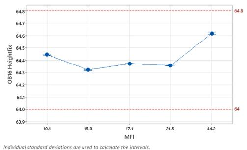
**Figure 13:** Outer barrel interval plot for height versus MFI.
