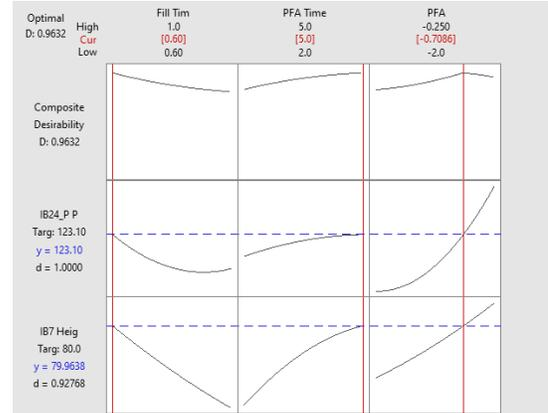
**Figure 10:** Response optimizer results for the inner barrel mold.
