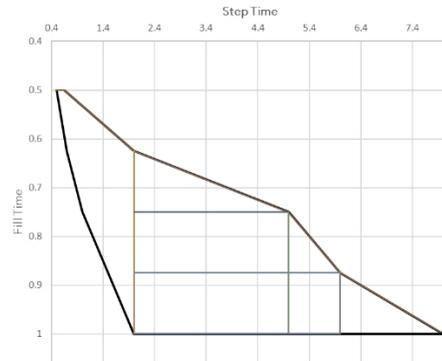
**Figure 2:** LECR process window with fill time versus step time.
