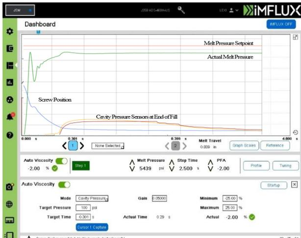
**Figure 1:** iMFLUX interface curve analysis.
