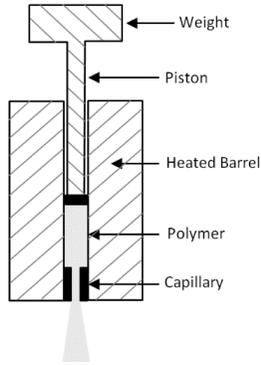
**Figure 9:** Melt indexer sample collection schematic.<sup>9</sup>
