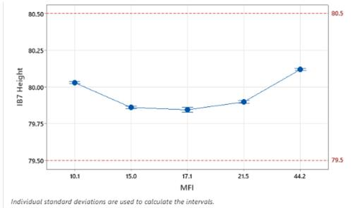
**Figure 12:** Inner barrel interval plot for height versus MFI.
