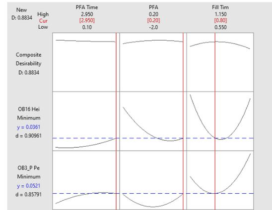
**Figure 11:** Response optimizer results for the outer barrel mold.
